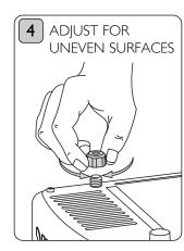
Your toaster is fitted with one adjustable foot which may be raised or lowered to compensate for unevensurfaces. The adjustable foot is located on the base of the toaster and is hexagonal in shape, rotate it to adjust the height.
